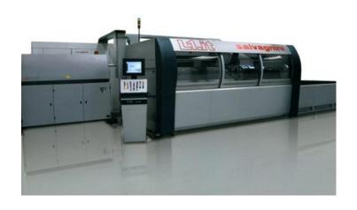
Laser cutting machinery with working area 3000x1500mm and cutting capacity up to 15mm thick.
