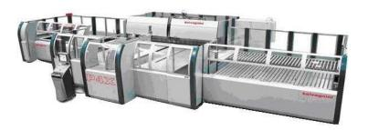
Automatic paneling machinery that allows the bending of thin sheet metal panels with high precision and repeatability of the pieces.
