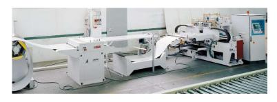
2 ski punching tape for thin sheets, which allows continuous processing of details of various types, especially panels, shelves and mantellature.
